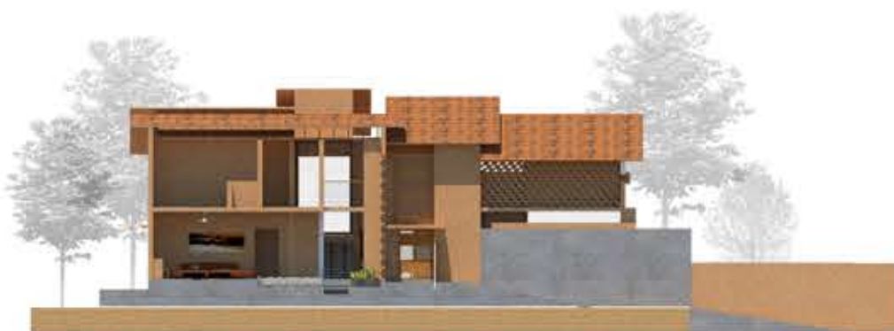
Section through the entry stairs
